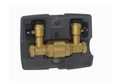
LK 322 CoolUnit is a valve combination that utilises the cold available in a system with a geothermal heat pump. By running the brine in the collector hose to a fan coil, you can cool your home with the cold naturally found in the ground. In addition, the borehole is recharged during the summer, which increases the performance of the heat pump.
