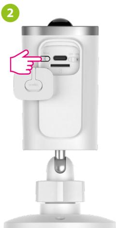
Make sure the camera is powered on. Then press and hold the button on the back of the camera for approximately 8 seconds, until the beep. The red LED on the front of the unit will then start flashing. The pairing mode is enabled.
