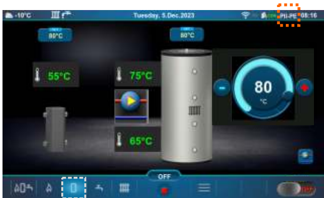
Accumulation (buffer) tank screen (PII-PE)
