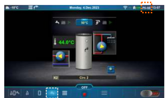
Domestic hot water (DHW) tank screen (PII-SE)
