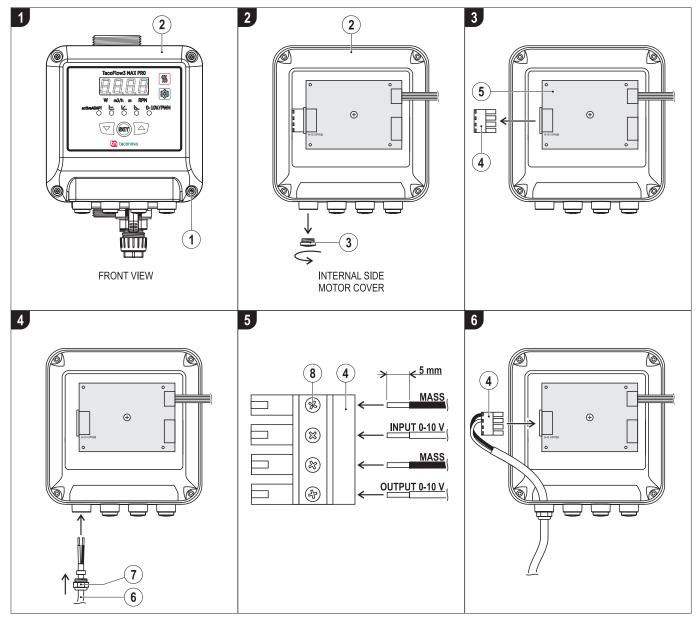
FIG. 11 (External connection for 0-10 V / PWM signal)
