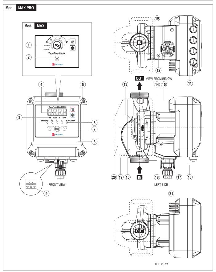
FIG. 3 (Name of the main components)
