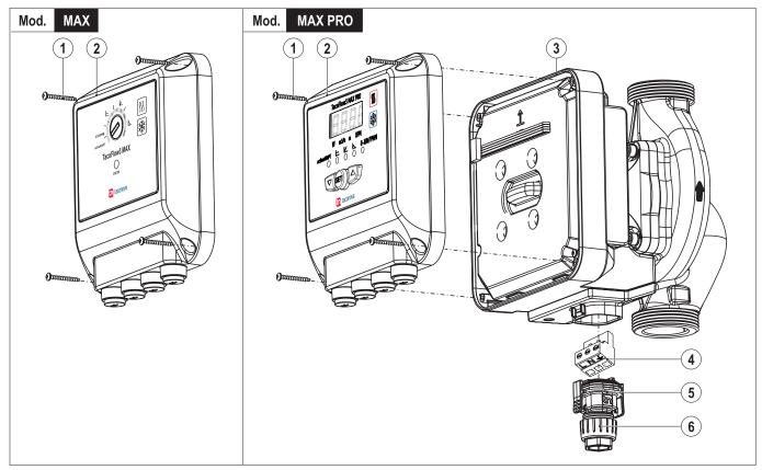
FIG. 4 (Name of the main components)
