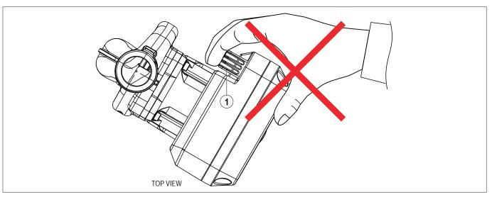
FIG. 6 (It is forbidden to handle the circulator holding it on the heat sink)
