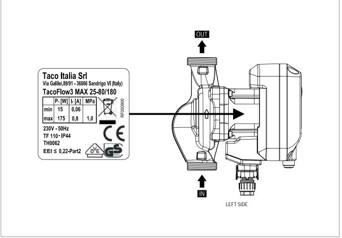
FIG. 1 (Data plate and CE marking)
