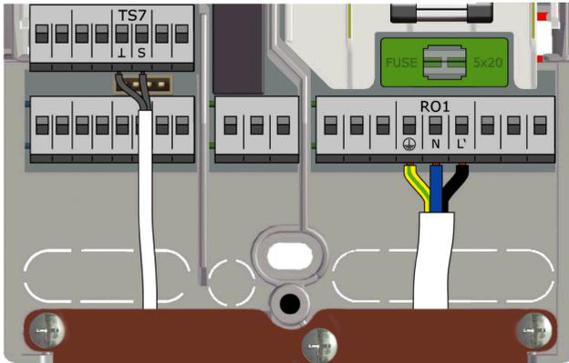
TS7/TS8: PWM-control signal for the high-efficiency pump
