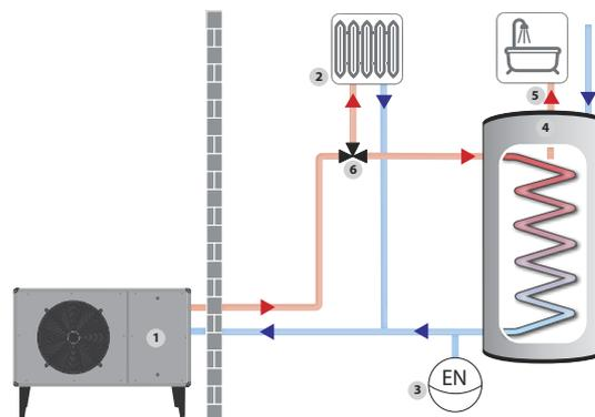
**Heat pump connected to a buffer tank and 3wv to the domestic hot water cylinder (dhw) 1-heat pump, 2-heating system, 3-expansion vessel, 4-buffer tank, 5-heating circulator pump, 6-dhw tank with coil, 7- dhw outlet, 8-3way valve**
