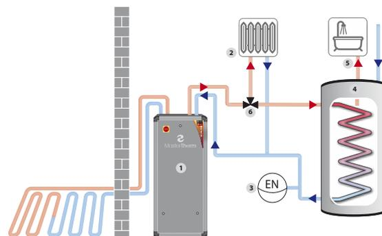
Heat pump connected to a buffer tank and 3wv to the domestic hot water cylinder (dhw) with desuperheater.
