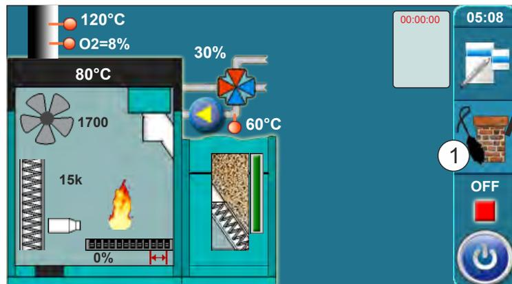
The factory set temperature that must be achieved to start measuring (except for conditions that can be changed - boiler power and time).
