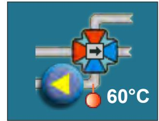
Motor device is opening the valve
