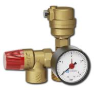
LK 924 / 925 SafteyGroup is a safety group for heating systems. The safety group contains manifold, manometer, safety valve and an air vent. 924 SafetyGroup has an automatic air vent with a float and 925 SafetyGroup has an automatic air vent with fibre discs. The manifold has two  $\frac{1}{2}$ " connections for safety valve and for example an expansion vessel, one  $\frac{3}{8}$ " connection for air vent.
