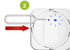
Make sure ZigBee gateway has been added to the Engo Smart app. Press and hold the function button for about 10 seconds until the blue LED starts flashing. The button will enter pairing mode.
