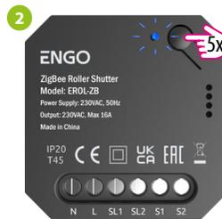
Make sure ZigBee gateway has been added to the Engo Smart app. Make sure the roller shutter is connected to the power supply. Blue LED should flash quickly. If not, press the button 5 times quickly or switch the controller's power off/on 5 times. The relay will enter pairing mode. In addition, device beeps when in pairing mode.
