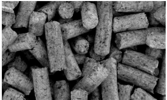
Poor-quality wooden pellets - dark with bark (with black dots)
