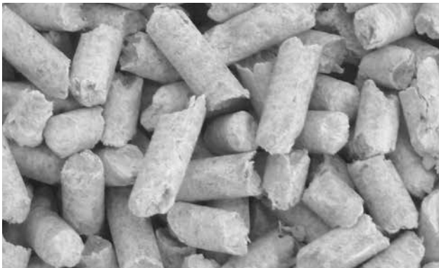
High-quality wooden pellets - white without black dots (bark)
