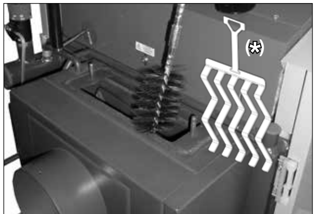
Sample cleaning of the flue way with a wire brush - upper lid Remove flue gas brake before cleaning. (* flue gas brake only DC30SPX)
