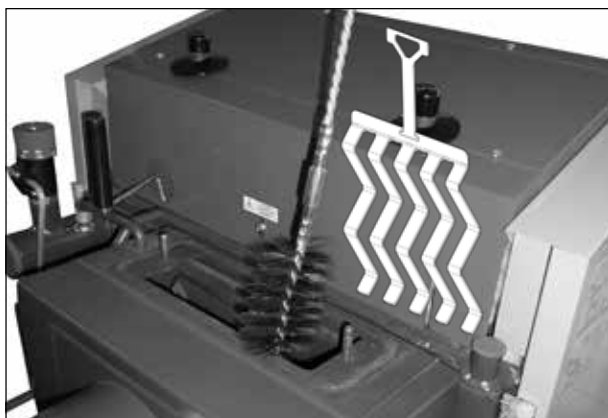
Sample cleaning of the flue way with a wire brush - upper lid Always remove the decelerator before cleaning.
