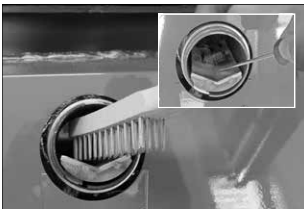
Example of cleaning the space above the ignition spiral plate
