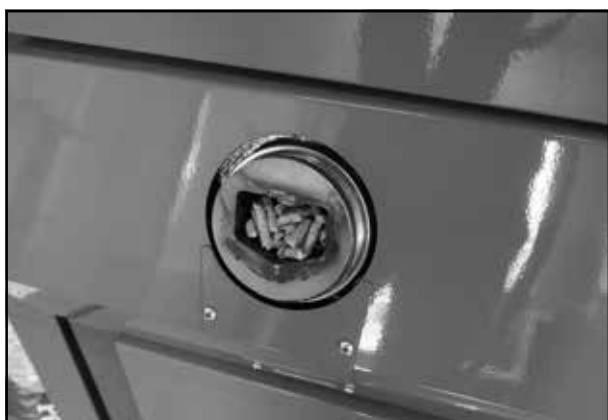
Pellets for ignition in the automatic ignition chamber
