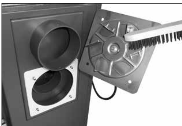
Sample cleaning of impeller and checking uprightness of vane on extract ventilator
