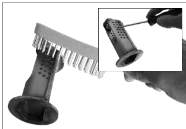
Example of cleaning the ignition chamber
