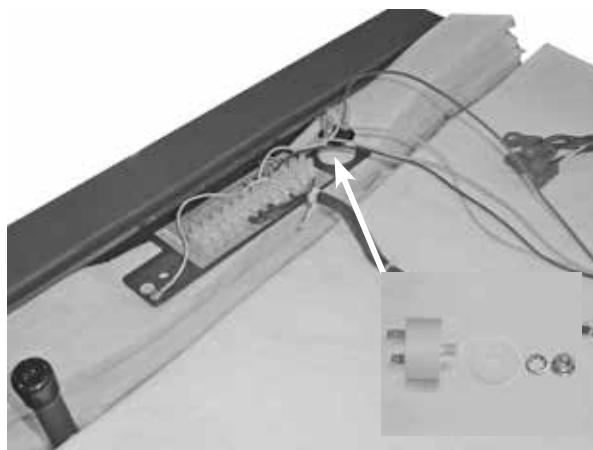
Capacitator for exhaust fan UCJ4C52 - 1µF
