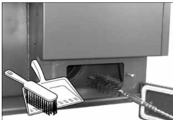
Sample cleaning of the flue way - bottom lid
