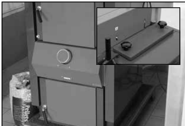
All doors and cleaning apertures closed
