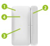
1. Sensor 2. Magnet 3. Function button Pressing for 8 seconds activates pairing mode and factory reset 4. LED diode
