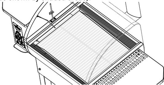
Direct heat will damage the meat probe wires. Always route the meat probes through ports on the side of the grill. Do not submerge wire in water. Not dishwasher safe.
