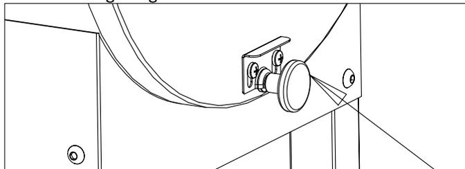
Never open the burner clean-out port when the grill is hot.
