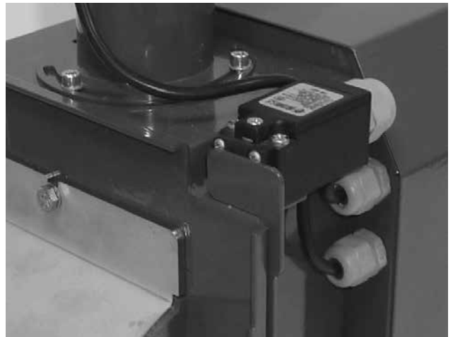
Fig. 8 - End switch with a special stop
