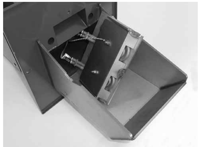
Fig. 4 - Disassembled plate with the ignition spirals
