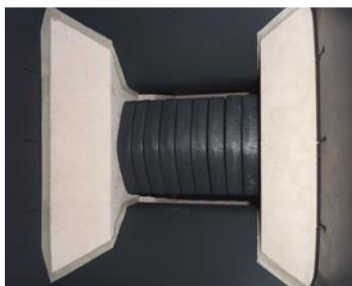
Cast iron grate allowing gasification
