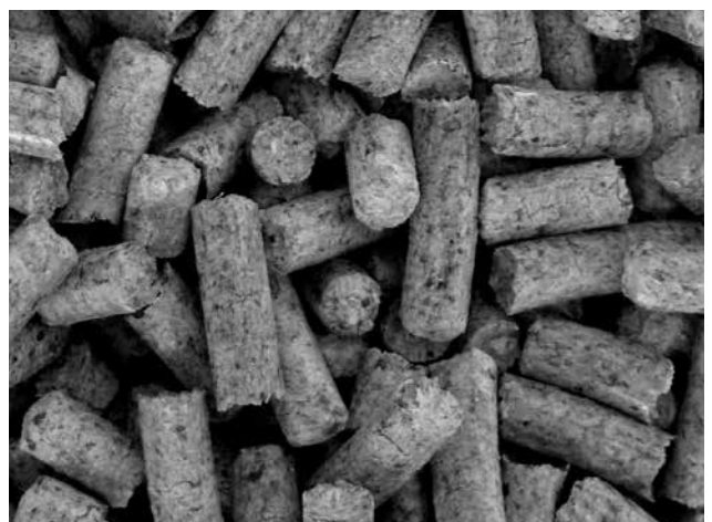
Fig. 18 – Poor-quality wooden pellets – dark with black dots (bark)
