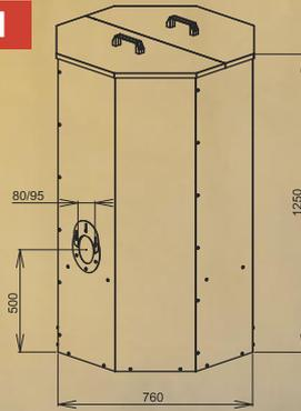
The **middle sized** silo is suitable for all boilers designed for smaller boiler rooms where larger silos cannot be used. It contains 325 kg of pellets which means approximately 1463 kWh (21 bags).
