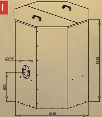
The **biggest** silo contains 650 kg of pellets which means approximately 2925 kWh (43 bags).
