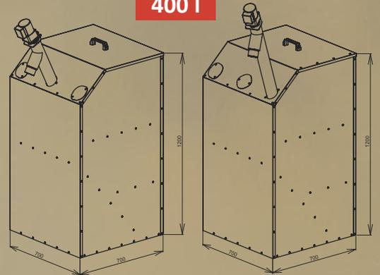
**AZPD/AZPU 400** – a set of 400 l silos with DRA25 conveyors – 1,3 m which is suitable for small boiler rooms. It can be placed beside the boiler to fit into smaller spaces. The 400 litre silo contains 260 kg of pellets which provides about 1170 kWh (17 bags).
