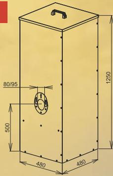
The **smallest** silo is suitable for all boilers designed for smaller boiler rooms where larger silos cannot be used. It contains 163 kg of pellets which means approximately 730 kWh (10 bags).
