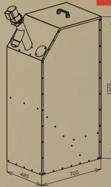
**AZPD 300** – a set of 300 l silos with DRA25 conveyors – 1,3 m which is suitable for small boiler rooms. It can be placed beside the boiler to fit into smaller spaces. The 300 litre silo contains 195 kg of pellets which provides about 880 kWh (13 bags).
