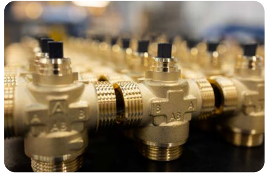
LK 525 MultiZone - made with recycled brass
